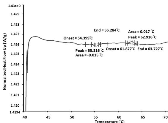
Fig. 2. Analysis of crystallization temperature by DSC at 61 °C
